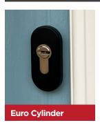
For this, we recommend a PTFE based lubricant for our Yale cylinders & a graphite powder for our Ultion cylinders. Rotate the key a couple of times in line with the normal locking function. Remove the key from the cylinder and wipe away any remaining lubricant to ensure it isn't transferred onto other objects. Less is more when applying to the components.
