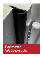
✓ Regularly checking the perimeter weather seal on your composite door is essential. Debris buildup or foreign objects can cause marks or damage to the door's surface. To prevent this, gently wipe around the seal with a soft, damp cloth and warm water. If you notice any part of the gasket is loose, simply push it back into position to ensure a tight, consistent seal when the door is closed. This will help maintain your door's appearance and performance. Every 6 months
